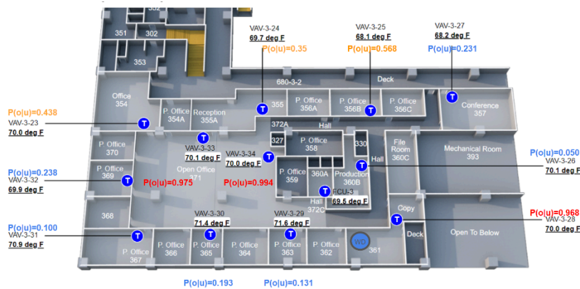
Figure 4: Floor plan showing thermostat locations in Student Financial Solutions and their probabilistic relationship to water dispenser usage.
